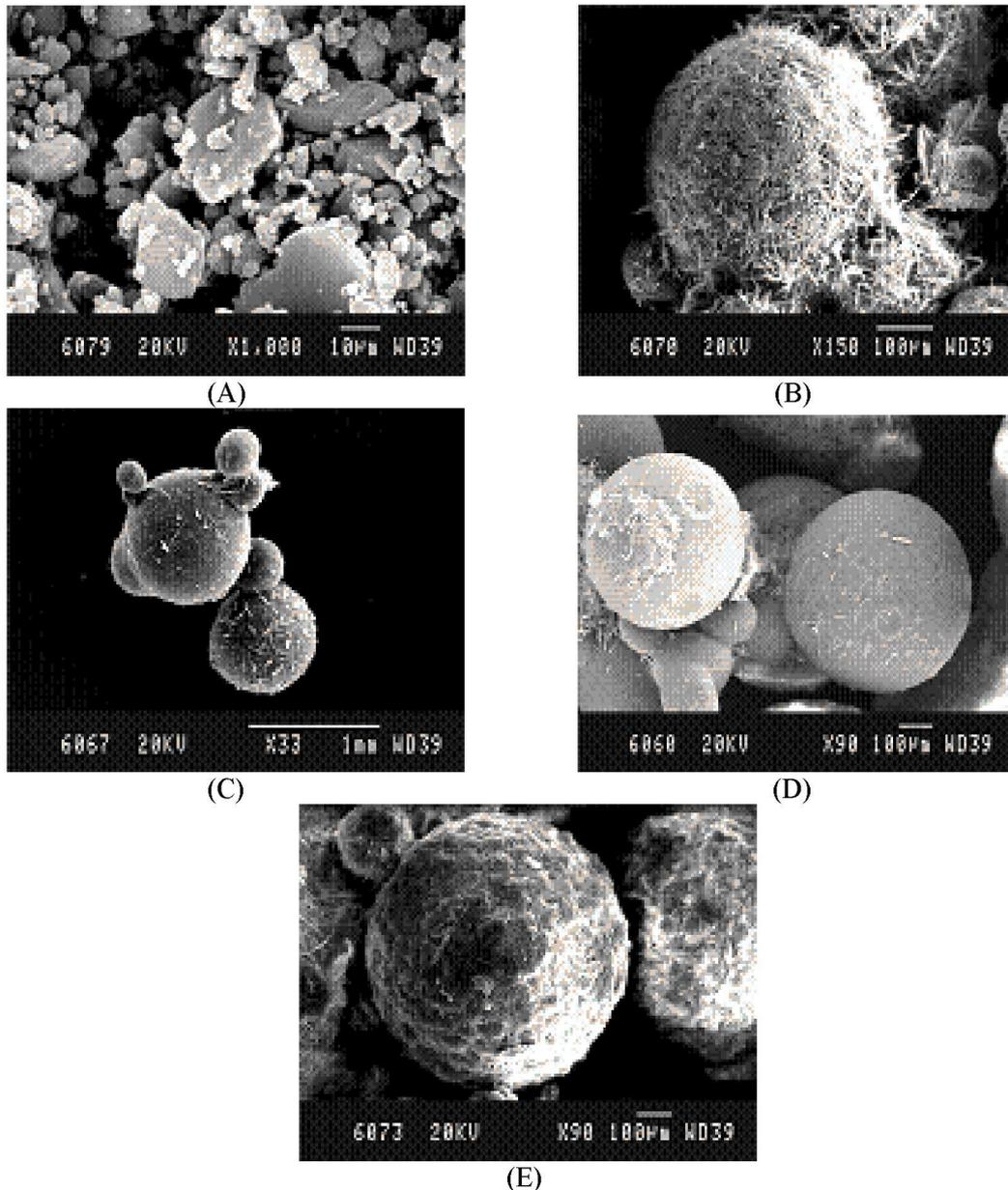
**Figure 1.** Scanning electron micrographs of indomethacin and indomethacin loaded ethylcellulose microspheres. Key, (A) Indomethacin drug particles, (B) F3, (C) F4, (D) F5, (E) F6.
