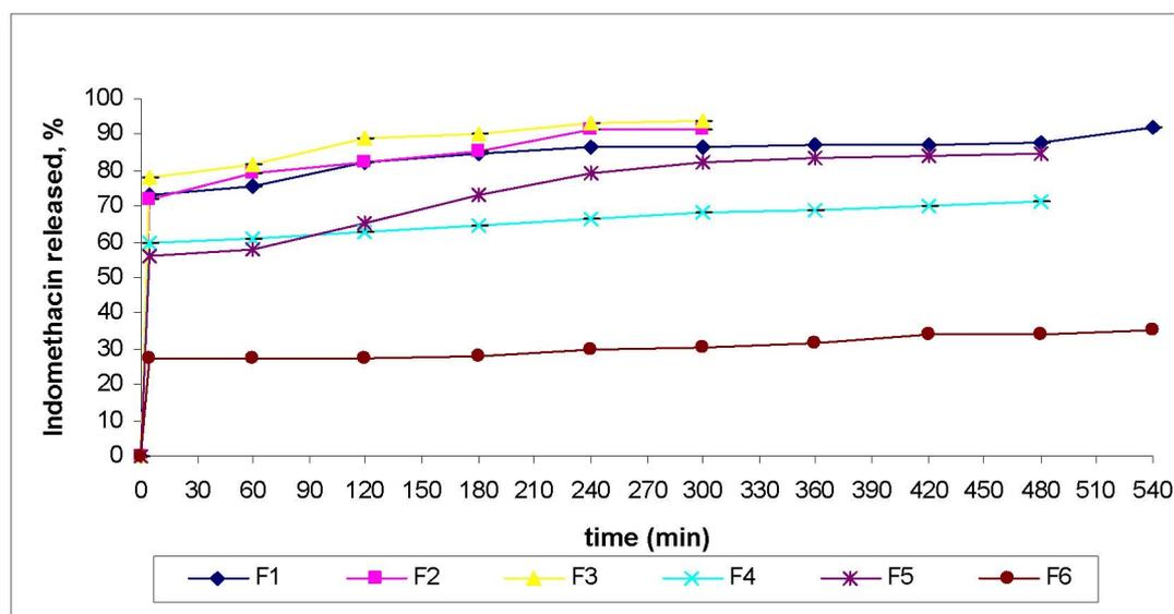
**Figure 3.** In vitro indomethacin release profiles in pH 7.2 phosphate buffer from different types of indomethacin-loaded microspheres.
