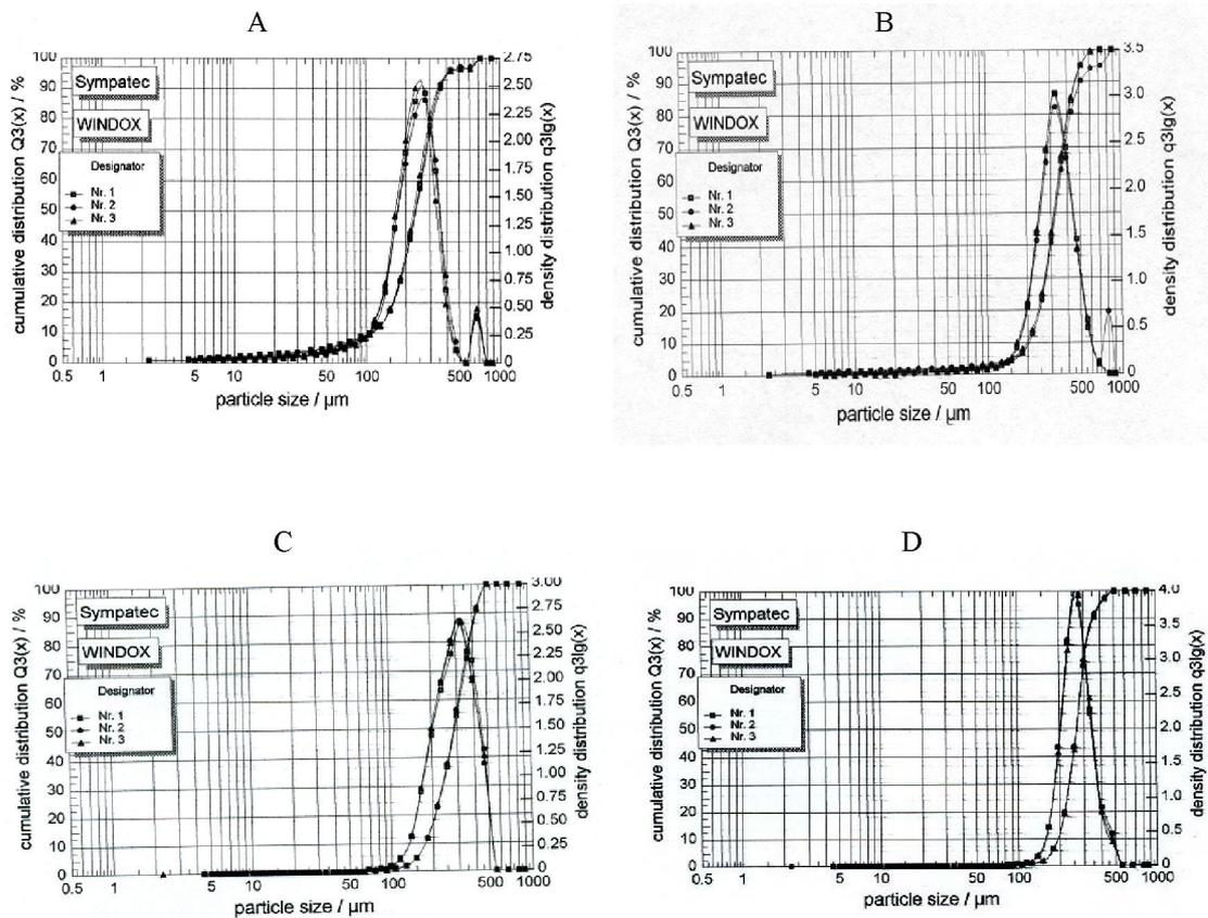
**Figure 2.** Laser diffraction patterns of particle size distribution of the microspheres with the average diameter  $\pm$  S.D. ( $\mu\text{m}$ ) ( $n=3$ ). Key; (A) F3,  $234.27 \pm 4.38 \mu\text{m}$ ; (B) F4,  $325.70 \pm 4.92 \mu\text{m}$ ; (C) F5,  $290.78 \pm 3.23 \mu\text{m}$ ; (D) F6,  $266.74 \pm 1.27 \mu\text{m}$
