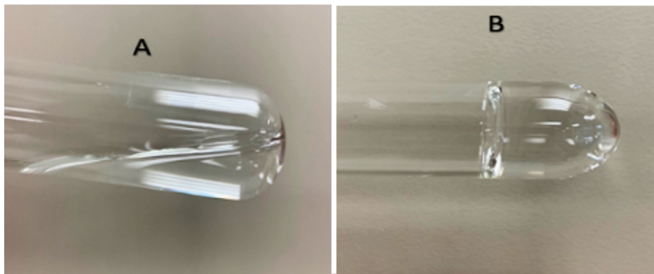
Figure 1. The figure shows the gels in solution form at 25 \text{ }^\circ\text{C} (A) and transformed into gels at 34 \text{ }^\circ\text{C} (B)
